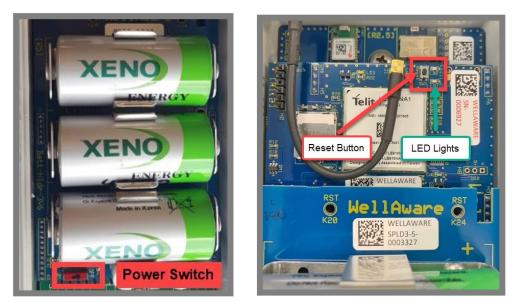
Once power is turned on for the Connect<sup>™</sup> you should then see flashing LED lights in the top right hand corner of the Connect<sup>™</sup> circuit board. If the lights do not flash, press the black reset button and wait a moment for the lights to flash. These lights indicate you have power. If your lights still do not flash, flip the power switch to off and then back to on again. If the LED lights still do not flash, please call your client success team at (210) 816-4600 (Ext. 2).
